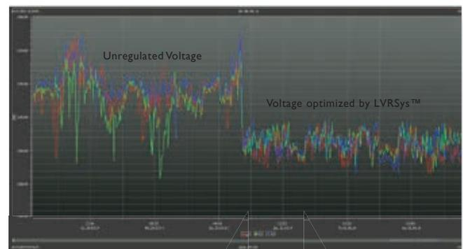
*Unregulated voltage compared to regulated voltage by LVRsyst<sup>TM</sup>*
