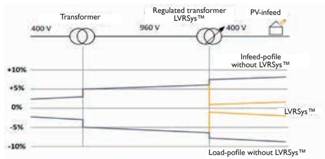
*LVRsyst<sup>TM</sup> - response model line regulator implemented as direct transformer regulator*
